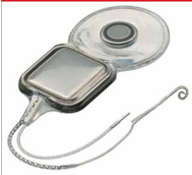
Figure 7: A Cochlear implant device, demonstrating the Nucleus receiver/stimulator package, straight ground electrode and precurved electrode array that is inserted into the cochlea. (Image courtesy of Cochlear Corporation.)
